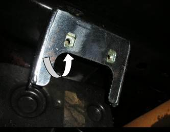
2. Place M8 cage nuts on inside of brackets. Place brackets on top of canister mount and between body of vehicle and secure using original hardware. Front canister mount shown.
