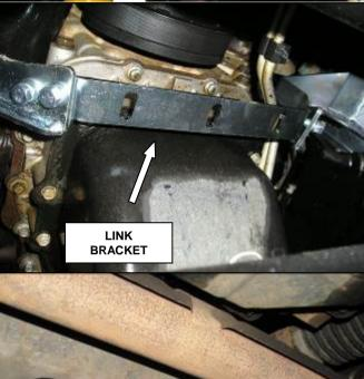
Place link bracket on top of engine mount brackets. Secure to engine mount brackets using M8 bolts, spring washers, flat washers and flange nuts. Leave all fasteners finger tight.
