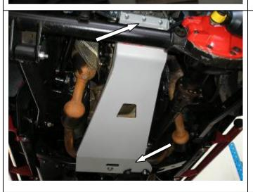
8. Place panel onto vehicle making sure it is placed between transfer case guard and chassis. Secure front using 3 x M8 bolts, spring washers, flat washers and flange nuts. Secure rear using original hardware and 1 M12 bolt, spring washer and flat washer supplied. When satisfied with the position tighten all fasteners leaving engine mount bolts until the very last. NOTE: If panel contacts exhaust use packers supplied on rear mounting position.
