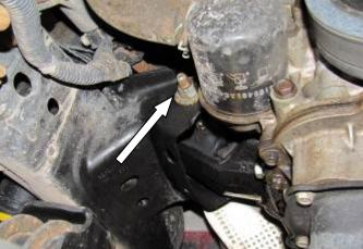
4. Loosen off both engine mount bolts leaving a gap of approximately 10mm between nut and chassis.
