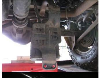
Remove and retain the three bolts securing the canister to the underside of the vehicle.
