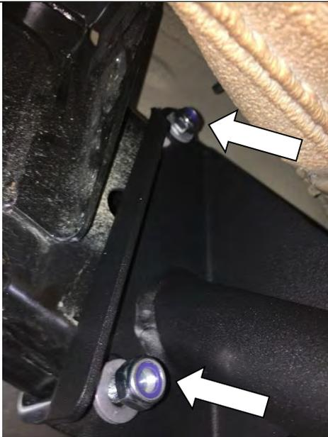
11. RHS Rear Only - Attach the rear mount of the step to the chassis using a U bolt, M12 flat washers and M12 nyloc nuts. **Leave loose at this stage.**
