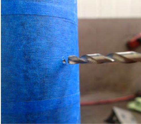
40. At the location of the centre punch mark, use a  $\text{\O}4\text{mm}$  (or similarly sized) drill bit to drill a pilot hole through the front face of the bull bar outer frame.
