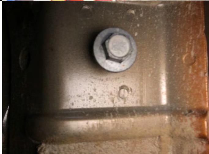
2. Refit the fasteners into the captive nuts in the vehicles body to seal against water ingress.
