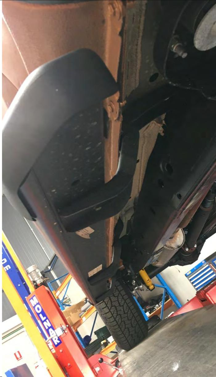
1. If fitted, remove the factory running boards/side steps retaining all fasteners (6 per step).
