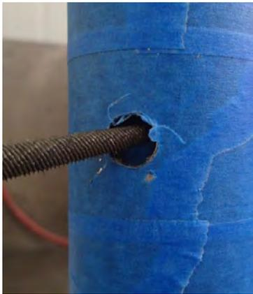
42. Using a small flat or half-round file carefully remove any burrs from the edge of the  $\text{\O}12\text{mm}$  hole.
