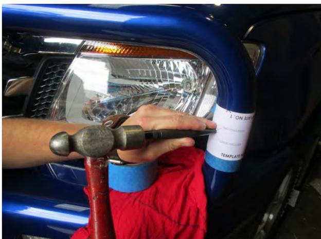
29. Using a centre punch, carefully centre punch the outer frame at the centre mark of "TEMPLATE 1".
