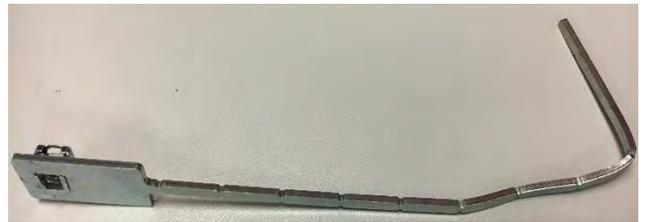
7. RHS & LHS - Bend the tail of the nut plate in accordance with the images below. Insert the nut plates through the hole located on the inner wall of the chassis.
