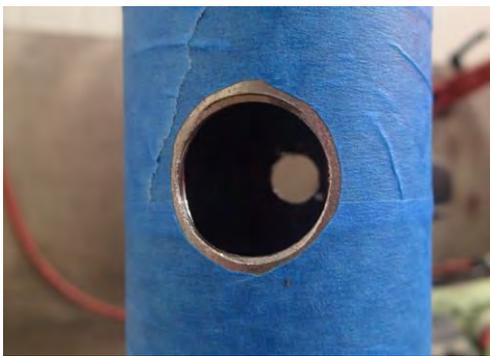
43. Remove all drill/file swarf and then clean and paint with rust preventative paint any exposed/bare metal surfaces left after drilling.
