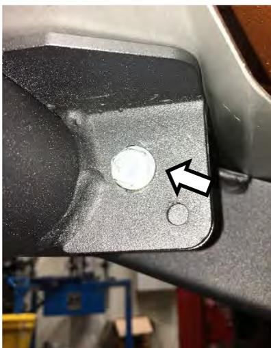
47. Tighten M8 bolt ensuring the slot and holes in the 6250024 1mm spacers (if fitted) are aligned with the holes in the step / front rail brackets.
