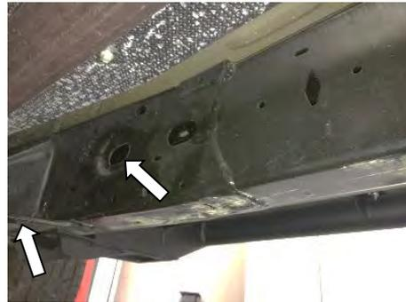
3. Fit the rubber plugs into the rear most ends of the side rails.
