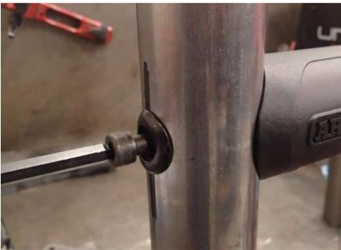
46. Install submerged bush and M10 bolt.
