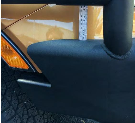
24. As a guide, set distance from top face of the bull bar wing to bottom of rail to approximately 85mm for correct set up.
