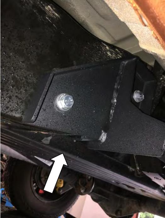
15. LHS Rear Only - Attach the rear of the rail to the chassis using M12 Bolts and M12 Flat Washers into the cage nut plates adjusted in the steps 4, 5 and 6. **Leave loose at this stage.**
