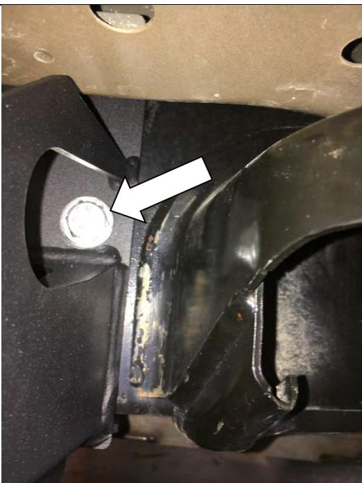
10. Attach the front mount of the side step to the chassis using M12 bolts and M12 Flat Washers into the cage nut plates adjusted in step 7. **Leave loose at this stage.**
