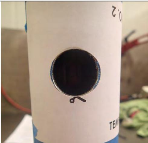
37. Carefully align "TEMPLATE 2" and centre over the Ø24mm hole. Wrap around the outer frame tube.
