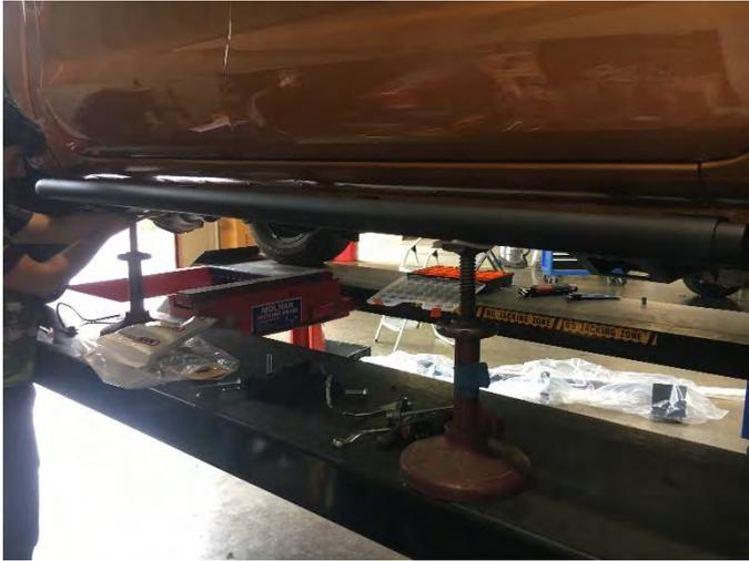
8. Place side steps up against outer chassis face, roughly in the correct position. Use adjustable axle stand or a second person to hold the steps in place. (RHS SHOWN).
