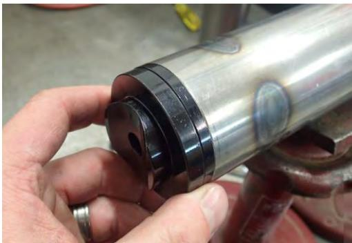
26. Swing the front rail outwards and away from the vehicle allowing installation of appropriate/selected spacer into gap between the front end of the front rail and the tube spigot. (5mm spacer illustrated in the image to the left).
