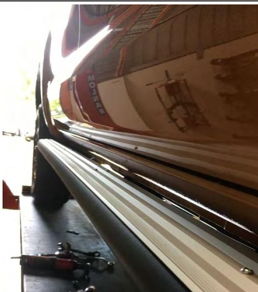
13. Adjust the rail so that it is level with the vehicle and tighten **all** fasteners to specified torque settings.
