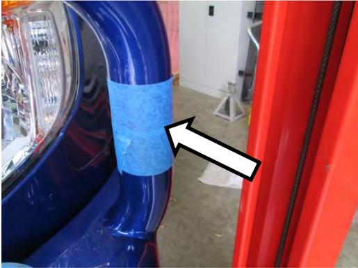
18. Use masking tape to wrap **1 x layer only** of tape around the bull bar outer frame to protect it from damage. Ensure masking tape is applied flat and without creases.
