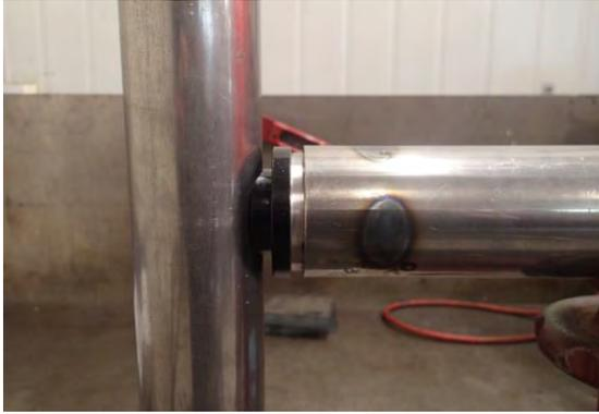
22. Hold front rail so that when viewed from the side of the vehicle the top tube is horizontal (**parallel to the ground**) and the side rail sits as desired against the side of the vehicle.
