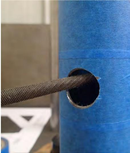
36. Using a small round or half-round file carefully remove any burrs from the edge of the Ø24mm hole.
